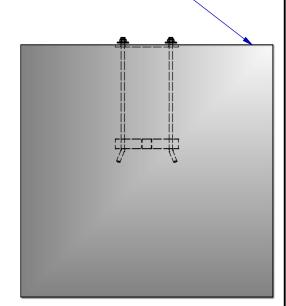
In case of a special ground surface, leave a 150mm space from the finished ground to the concrete.
