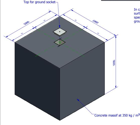
In case of a special ground surface, leave a 150mm space from the finished ground to the concrete.
