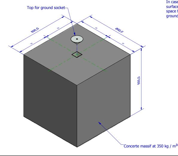
In case of a special ground surface, leave a 150 mm space from the finished ground to the concrete
