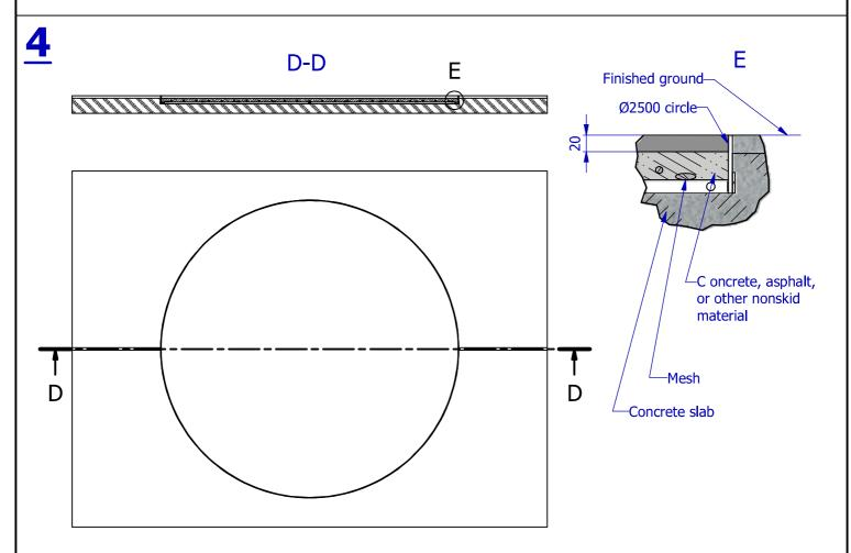
After mesh has been installed, fill the circle up, with concrete, till you have a flate surface at 20mm from the upper part of the circle
