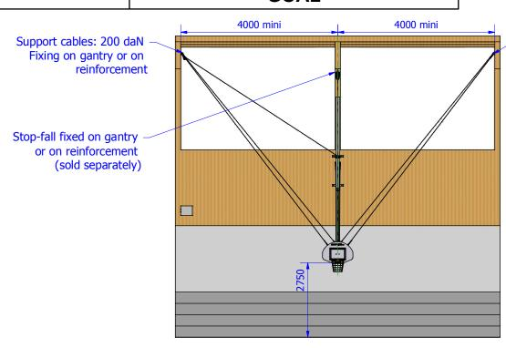
Support cables: 200 daN Fixing on gantry or on reinforcement
