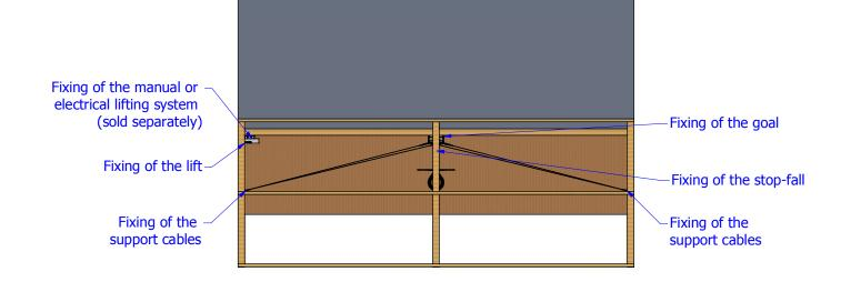
The different efforts of the attachment points of the goal on the frame (included return cables and lifting system) are subjected to the verification by a BET structure or a carpenter following the norm NFS 52-400.
