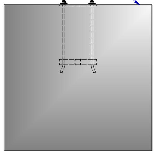
In case of a special ground surface, leave a 150mm space from the finished ground to the concrete.
