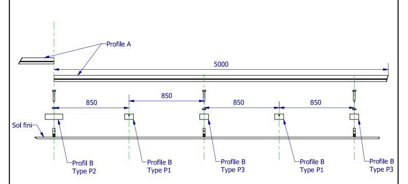
Piece 1 (Profile B, type P1) --> 3 fixed pieces joining the profil A by mens of clinching.
